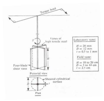
Shear failure occurs over the surface and the ends of a cylinder having a diameter *D*, equal to the diameter of the vane.
