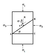
The critical stress values generally occur on planes normal to the intermediate plane. Consider a plane AB of unit width perpendicular to the plane of the paper, inclined at  $\theta$  to the major principal plane.
