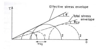
In normally consolidated clays there is a tendency towards volume decrease under undrained conditions during shear (that is, for pore water to escape). If this volume change is not allowed to occur, positive pore water pressures develop. Consequently, effective stress Mohr circles lie to the left of total stress circles (i.e. effective stress and total stress failure envelopes for the normally
