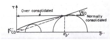
This is similar to **CU test** except that as deviator stress is increased, drainage is permitted. The drainage valve is kept open in both the phases of the test. During the shearing phase, the rate of loading must be slow enough to ensure no excess pore water pressure develops. Therefore,
