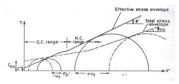
In overconsolidated clays there is tendency towards volume increase under undrained conditions during shear. If this volume increase is no allowed to occur, negative pore water pressures develop. Consequently, effective stress Mohr circles lie to the right of total stress circles (i.e. effective stress > total stress). The failure envelope for an overconsolidated clay is not a straight
