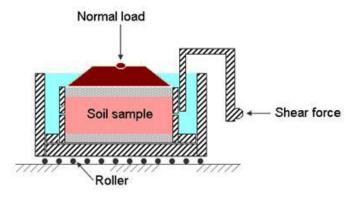
The test is carried out on a soil sample confined in a metal box of square cross-section which is split horizontally at mid-height. A small clearance is maintained between the two halves of the box. The soil is sheared along a predetermined plane by moving the top half of the box relative to the bottom half. The box is usually square in plan of size 60 mm x 60 mm. A typical shear box is shown.
