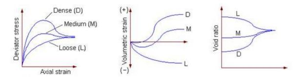
For the dense sand sample, the deviator stress reaches a peak at a low value of axial strain and then drops down, whereas for the loose sand sample, the deviator stress builds up gradually with axial strain. The behaviour of the medium sample is in between. The following observations can be made:
