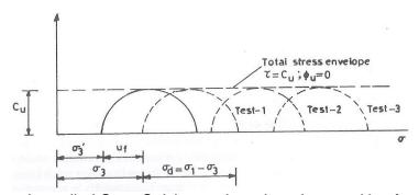
In this test, cell pressure during the consolidation phase is applied without allowing drainage. Then keeping cell pressure constant, deviator stress is increased to failure without drainage. Thus, the drainage valve is closed throughout the test. This is a total stress test and does not usually intend measuring the pore pressures. It is
