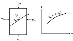
For the soil element at failure, principal stresses at failure are  $\sigma_{1f}$  and  $\sigma_{3f}$  and the normal and shearing stresses on the failure plane are  $\sigma_{ff}$  and  $\tau_{ff}$ .
